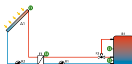
External heat exchanger, zone loading, intelligent valve control, heating return increase
